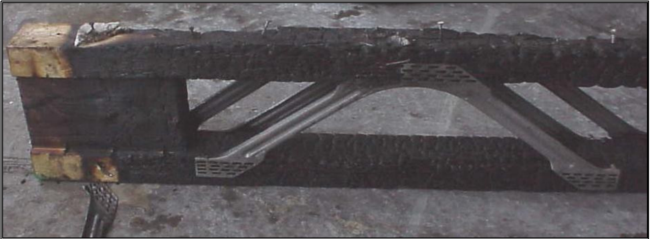
Photograph 9. Joist after test, showing extent of damage (the other joists were in a worse condition than this one, but had fallen into the furnace).
