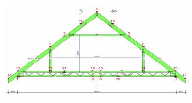
The GN Roof & Truss software has speedy macros to design and detail these requirements using standard construction elements of solid timber and GN plates but it is now becoming quite common to incorporate Ecojoist as the bottom chord of the truss. The design office of Gang-Nail Systems have the ability to design the Ecojoist as the bottom chord within the attic truss within Roof & Truss but before any further development work is commenced
